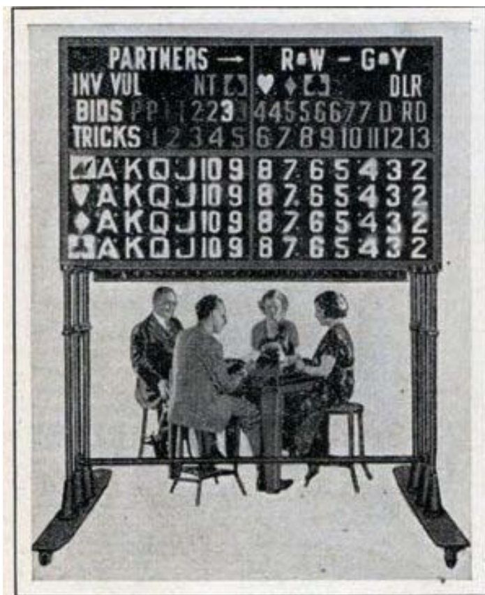
Bridge players from any part of country can sit in at tournament by watching this electrical annunciator board. Key on the bridge table are operated to indicate plays on board
